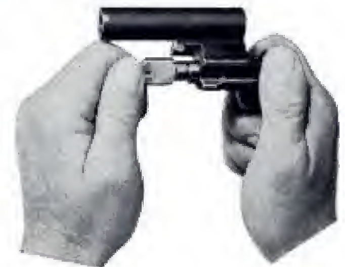
Fig. 35 Stripping the bolt assembly
